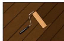
Apply a uniform even coat. Stain the full length of boards, keeping a wet edge. One coat is sufficient for most applications. On decks, wipe up any excess product that is not absorbed within 5 minutes to prevent tackiness and surface sheen.
