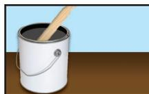
Stir well initially and during use. Intermix all containers of the same color to ensure uniform appearance. Cover plants, grass and concrete to protect from spills.
